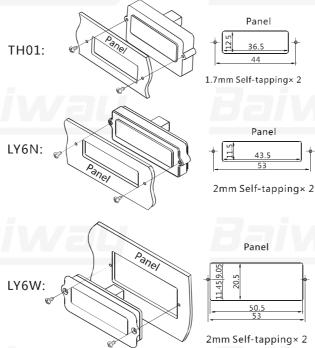
**LY6W:** First, open one rectangular orifice and two screw holes on the panel of the equipment. Then install the tester from the front of the panel, and put the shell of tester into the
